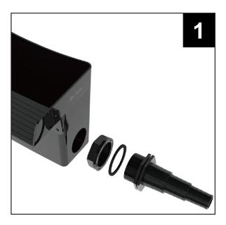
Insert universal hose adapter through side hole. Place O-ring inside of Matala<sup>®</sup> Minifall and over the threads. Hand tighten nut.
