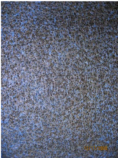
Figure 8 – Pressure Drop Caused by Grease at Lower Media
